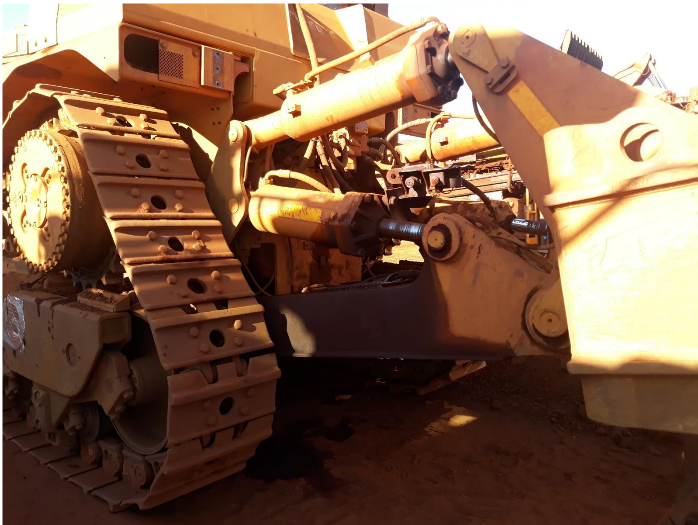
LH Rear view showing Oil Leak from Banlaw fitting above LH Ripper Lift Cyl
