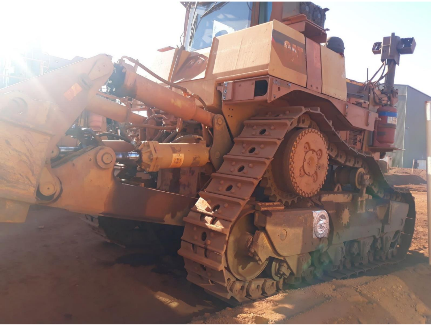
Rear View – Tilt and Lift Cyl seals weeping
