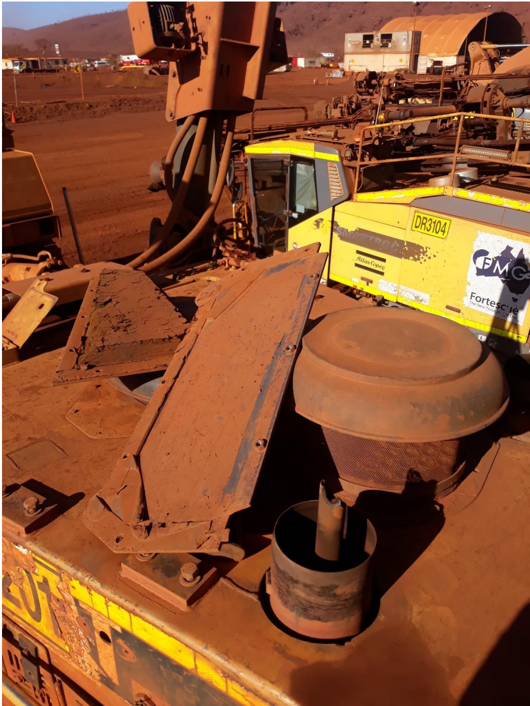
Top Engine cover with Exhaust stacks removed
