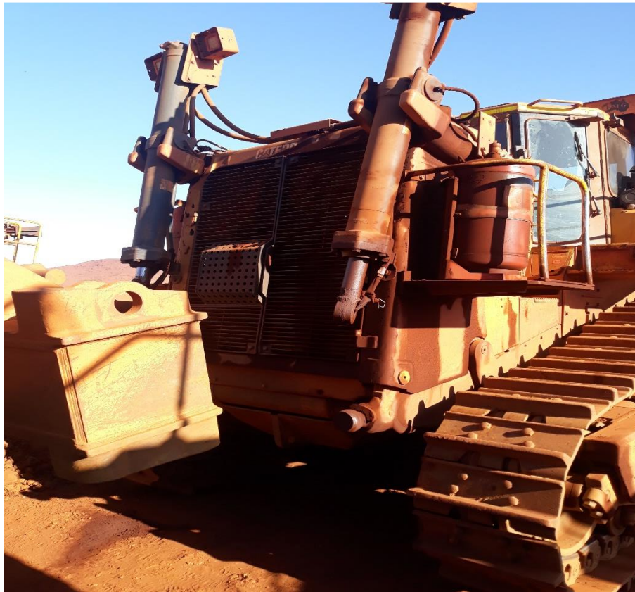
Front View showing 2 x Lift Cyl Leaking
